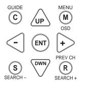
**MENU/OSD button:** Press to display the SYSTEM STATUS screen. From the SYSTEM STATUS screen, press the ENTER button to display the MAIN MENU screen which has links to all other menus. If a menu is already visible, push this button to cancel the display. The MENU button on the front panel provides the same function.
